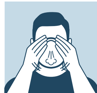
PERFORM A FIT CHECK: PLACE HANDS OVER THE RESPIRATOR AND EXHALE, ADJUST IF THERE ARE LEAKS
