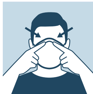
PRESS THE METALLIC WIRE TO FIT THE SHAPE OF YOUR NOSE AND FACE
